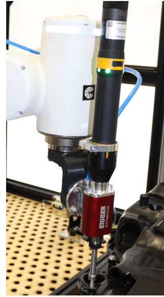
Fig. 12. Mounted SPATZ04 system screwing the housing of an iMOW ® .
